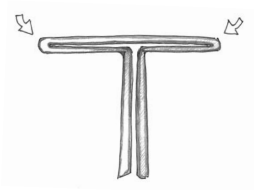
In this cross section view of a T-fold the fold edges are marked with arrows. Most foldforms have fold edges.
